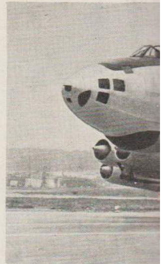
Left, Major L. E. Gunter, and Capt. R. R. Barto and A. T. Brent, of the 369th Sqn., enter their B-47. Note their helmets, visors and extra-bulky parachute packs. Right, this view of the B-47 shows the marked ground anhedral of the wing. The bulge beneath the cockpit houses radar gear, while in the extreme nose is an optical bomb sight. Below, pilot and co-pilot in their long cockpit, with the radio compass aerial in between.
